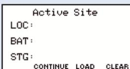
To select a site before testing, select Load|Access Setup Data. Press the arrows to step to a site, then press Select. If "Active Site" displays the correct site name, press Continue to return to the main menu.
