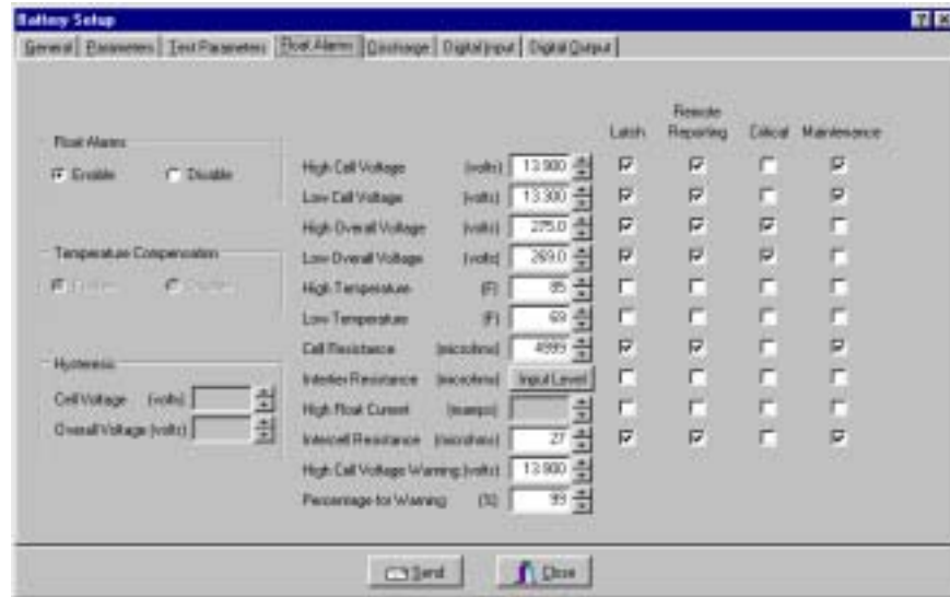
Figure 26. Battery Setup - Float Alarms (BDS)
