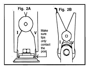
NOTE: Do not connect to the stainless steel bolt heads to make this measurement.
