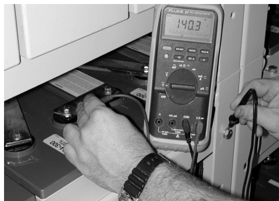
Fig. 4b: AC voltage to ground 140 v rms
